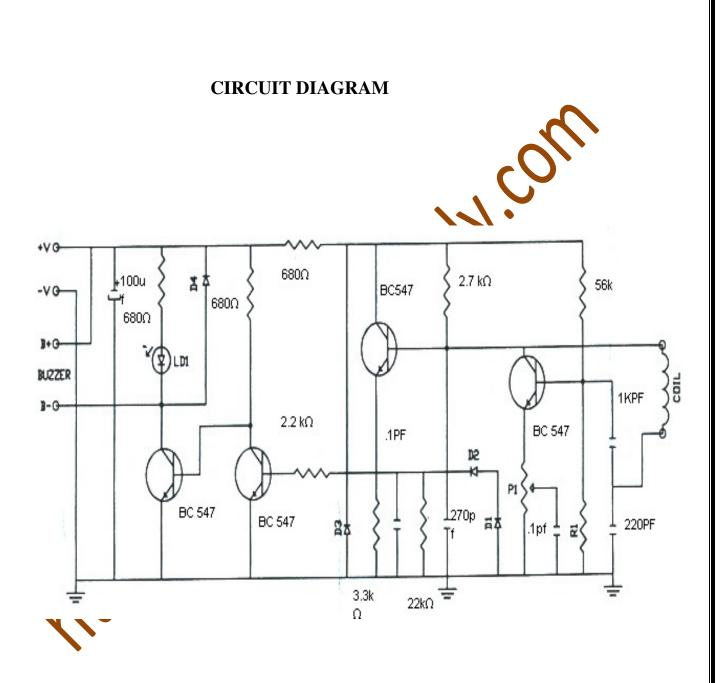
D1,2,3,4 -IN 4148L formula ra multilayer air -core type coil me coil . L=  $0.8r^2N^2/(6*r+9*l+10*d)$
